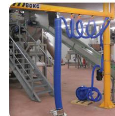
**Sack tube lifter** for an effortless loading of the machine. The rate is guaranteed with maximum ergonomics
