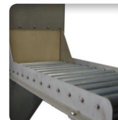
**Roller conveyor** to feed the machine
