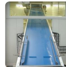
**Belt conveyor**, vertical or inclined. It integrates detection cells to adjust the flow rate of the machine
