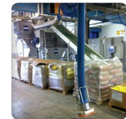
▶ Tube lifter to lift sacks effortlessly for an ergonomic working station (option)
