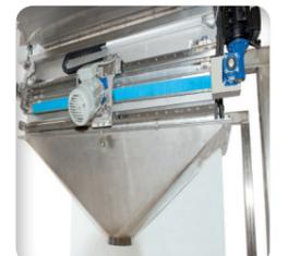
**Vibrating chute** allows to channel the product flow for introduction into the process upstream
