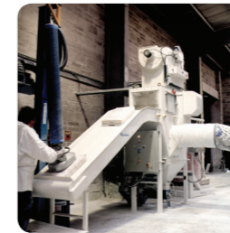
Sack tube lifter and belt conveyor
