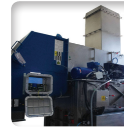
Dust collector system to vacuum fine particles.
