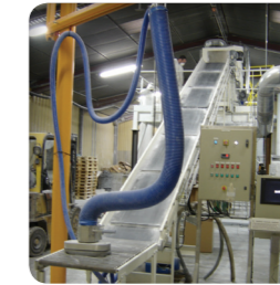
Vacuum lifter for sacks for effortless handling and improvement of the production
