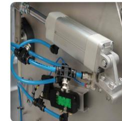
▶ Pneumatic cutting cylinder with accumulator for more efficiency cutting
