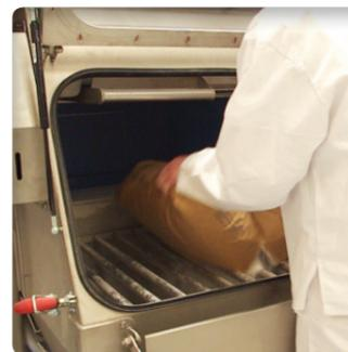
▶ Shaking of the sack without effort and without heavy lifting of the sack. The operator does not need to return the bag.
